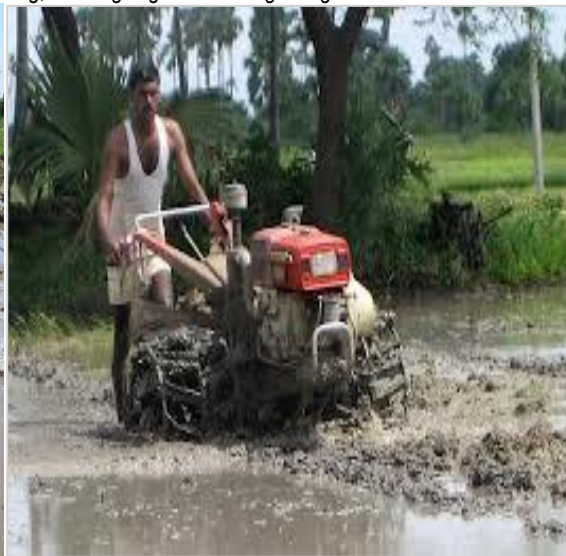
Fig. 9. Puddling of field using power tiller
